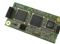
Plug-in to the AR5001D Approx. size 125 x 50mm
