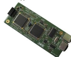
Plug-in to the AR5001D Approx. size 100 x 50mm
